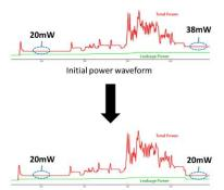
Power waveform after fixing power bug
